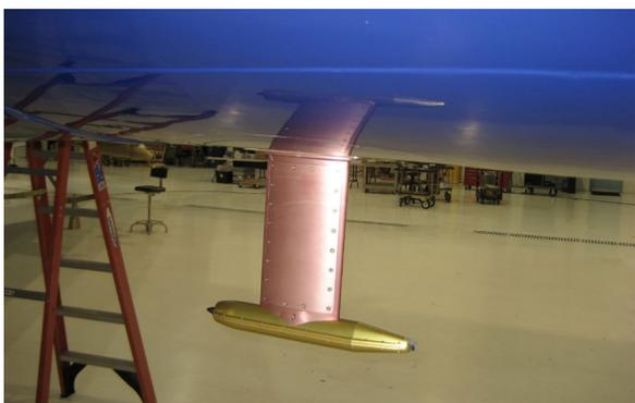
**Greenhouse Gas Sensors:** aircraft-mounted sensor, measuring the types and quantities of different greenhouse gases
