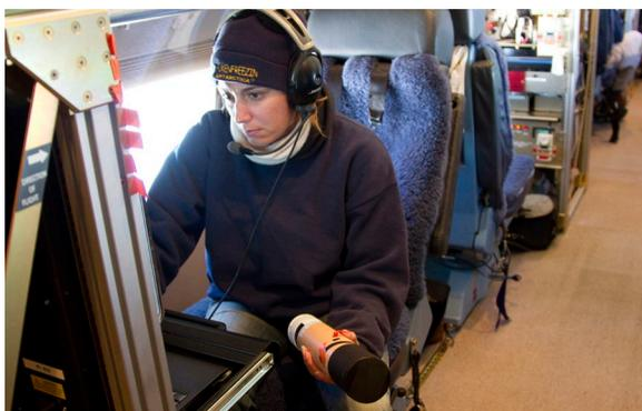
**Droppsonde:** measuring temperature, pressure, humidity, wind speed & direction, dropped from aircraft to sea surface; about the size of a tennis ball canister
