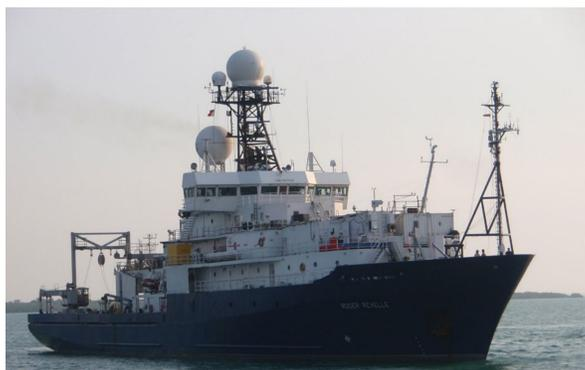
**Ship-based Radar:** looking at cloud particles (mounted high on the ship in a protective “ball”)
