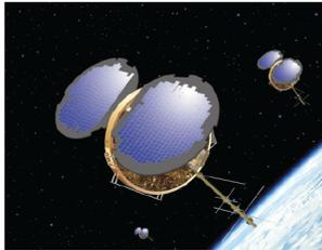
A COSMIC satellite monitors how GPS radio signals bend in the atmosphere.
