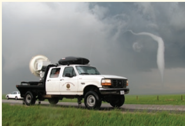
A W-band radar deployed by the universities of Oklahoma and Massachusetts captured the end stages of the 5 June 2009 tornado in Goshen County, Wyoming.
