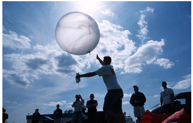
Weather Balloon :: attached instrument measures temperature, pressure, humidity, wind speed, & wind direction profile from the ground up to about 60,000'
