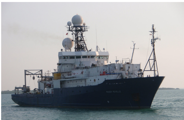
Ship-based Radar :: looking at cloud particles (mounted high on the ship in a protective "ball")
