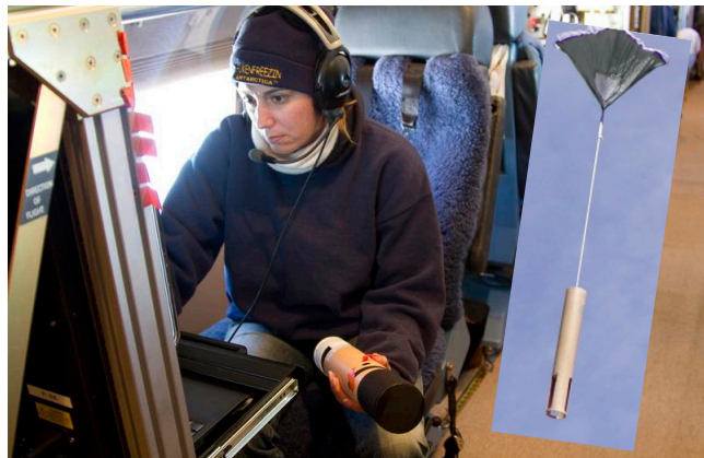
Dropsonde :: measuring temperature, pressure, humidity, wind speed & direction, dropped from aircraft to sea surface; about the size of a tennis ball canister
