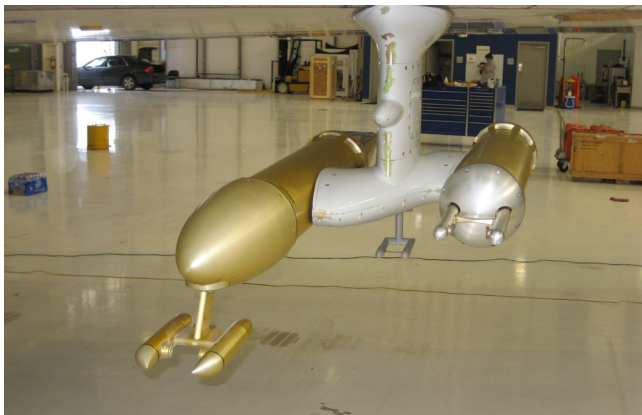
Cloud Droplet Sensor :: aircraft-mounted sensor measuring cloud droplet size and distribution
