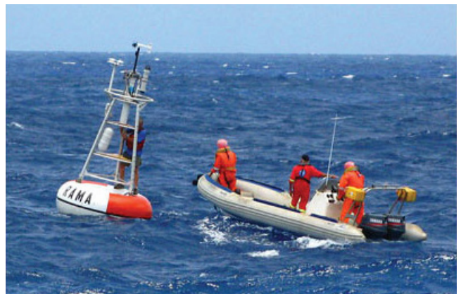
Buoy System :: located throughout the Indian Ocean at fixed locations, sensing sea surface temperature
