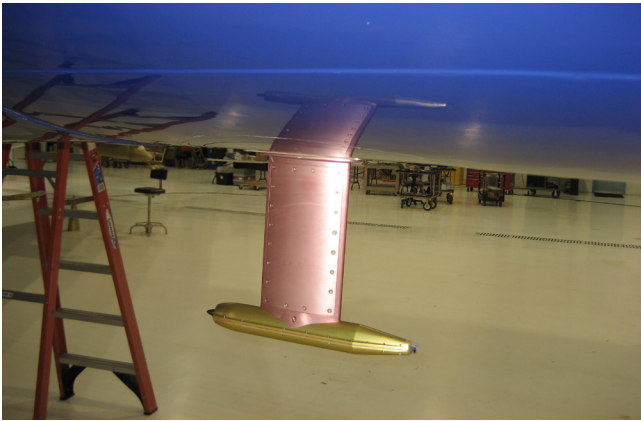
Greenhouse Gas Sensors :: aircraft-mounted sensor, measuring the types and quantities of different greenhouse gases
