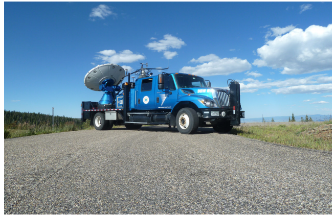
Truck-mounted Radar :: radar mounted to the back of a truck so it can easily drive close to a storm to observe winds
