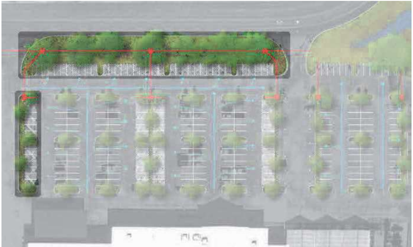
CH7-48: This image provides an example of how the required perimeter planting area might be designed and constructed to integrate the landscaping and stormwater management together.
