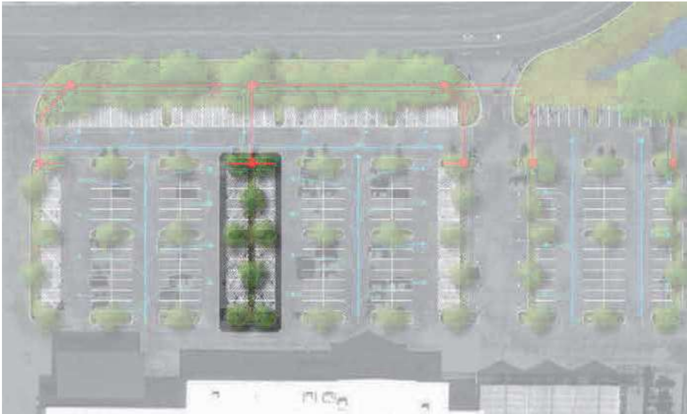
CH7-50: This image provides an example of how the required planting median area might be designed and constructed to integrate the landscaping and stormwater management together.
