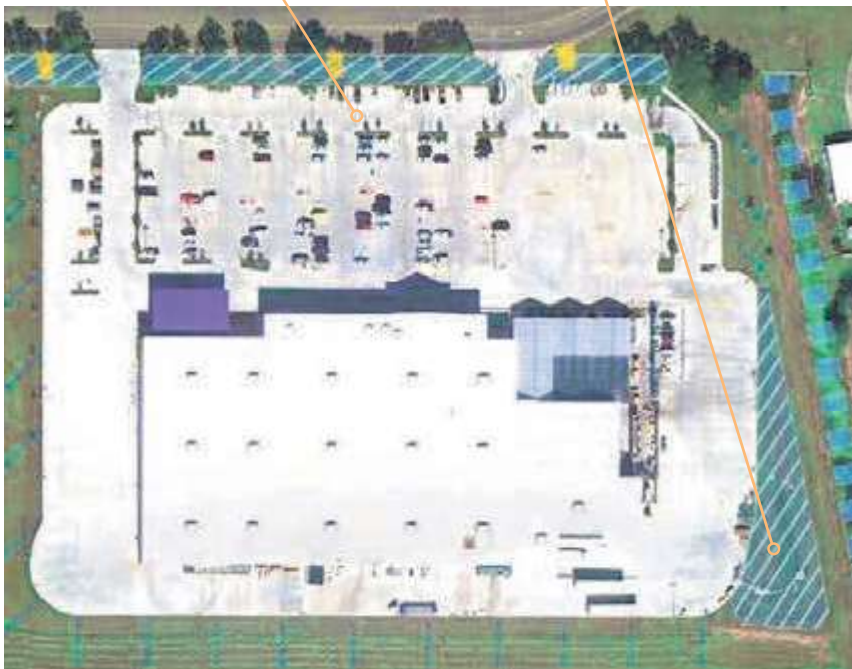
CH7-40: The parking lot of this big box is typical of new parking lots built throughout coastal Louisiana. There is limited landscaping and nominal stormwater management measures. This is an example of a good result for a community with no rules for how parking lots and stormwater should be managed.
